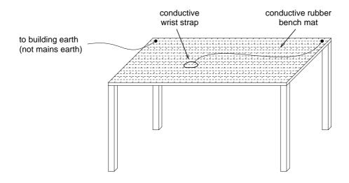
Figure 1.2 Typical Anti-static Bench Set-up
