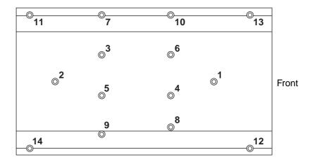
Figure 2.3 Receiver/Transmitter Bottom Cover Screw Tightening Order
