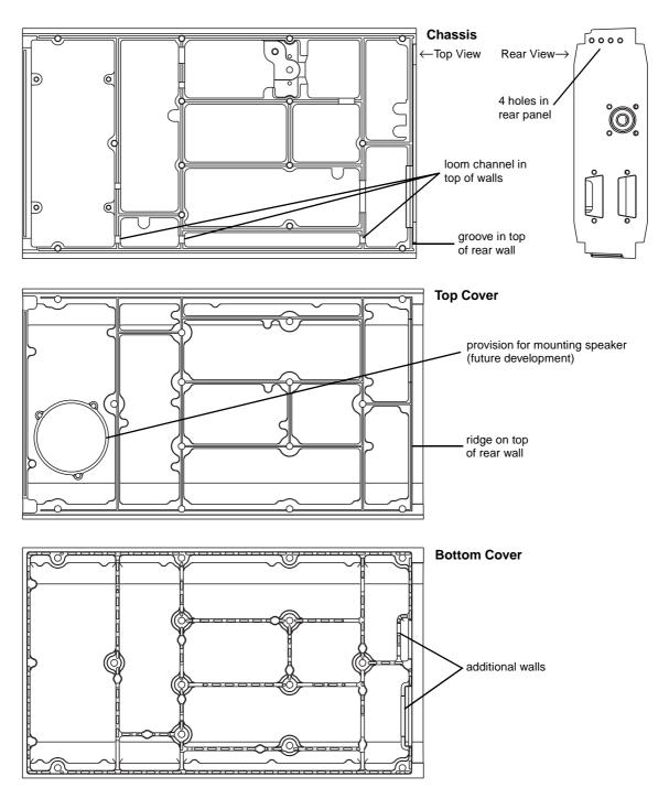
Figure 2.4 Identification Of New-Design Chassis & Covers
